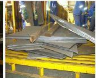
Stack of blade skins after incident
