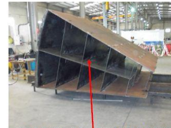
Photo 1- Section, parts of a rotor where worker was working
